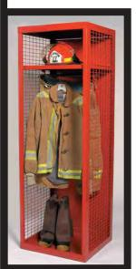
tion of locker contents. The base model is constructed of a 16-gauge steel frame, back, top and bottom, with our tough 2" x 1", 10-gauge wire mesh welded onto the side wall frames. A heavy load capacity, 16gauge steel shelf is mounted 12" from the top of the locker with two coat hooks and a coat rod secured below.
