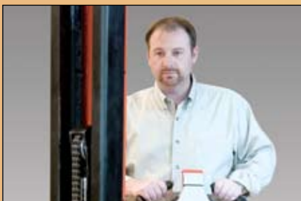
Offset handle and narrow mast design (62" mast only) provide a clear view with no "blind spots"
