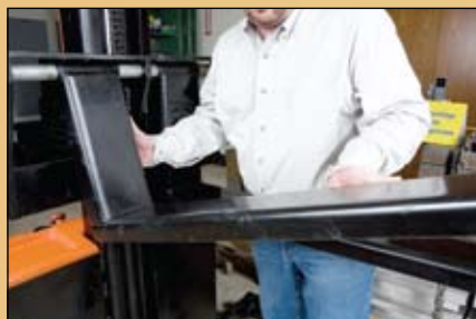
Adjustable fork carriage allows forks to be quickly repositioned to best accommodate loads (straddle only)
