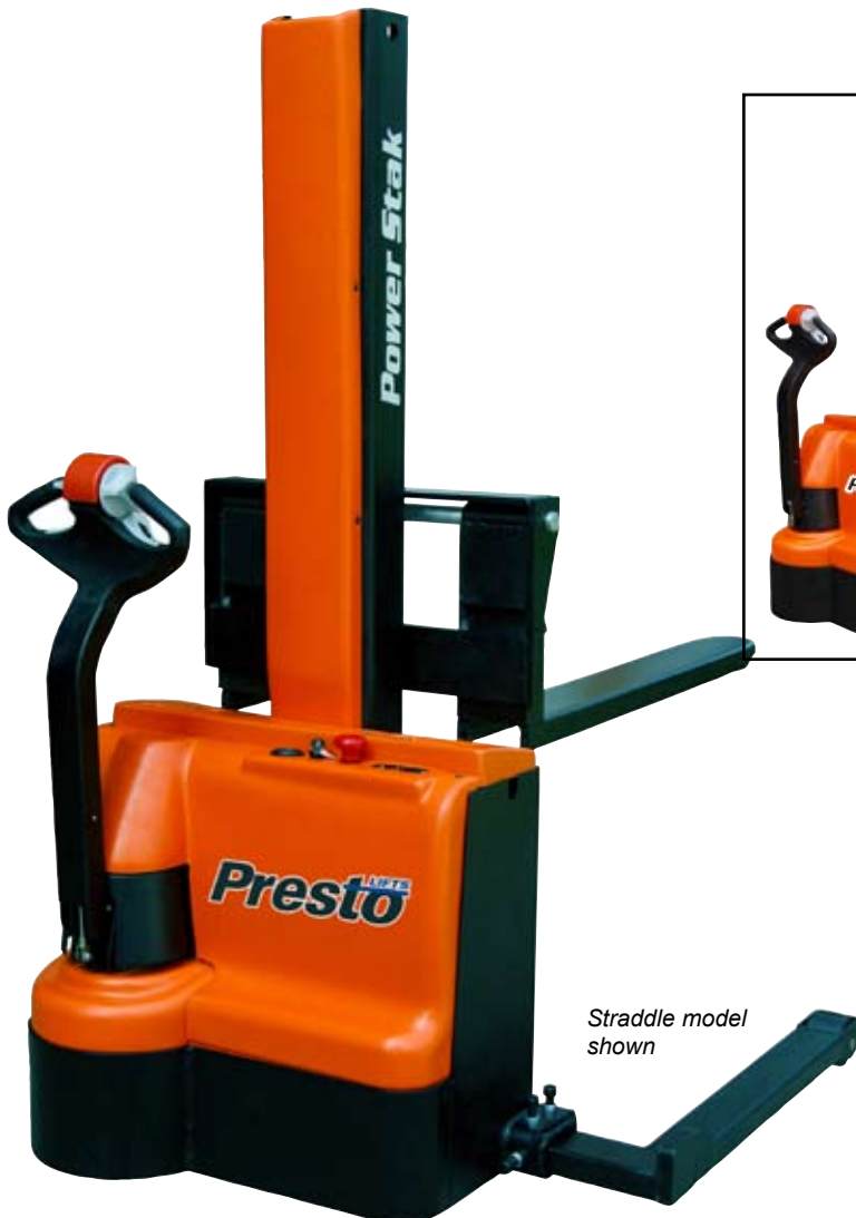
Adjustable fork carriage allows forks to be quickly repositioned to best accommodate loads (straddle only).
