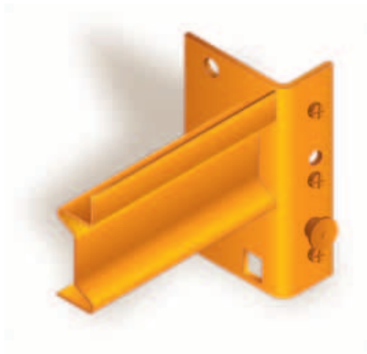
ZS Beams-U65 = 14 ga For use with wire decking
