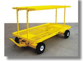
Shelves are available in a variety of sizes with either expanded metal or solid bottoms.
